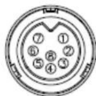
Conn. 1 Pin Assignments Front View
